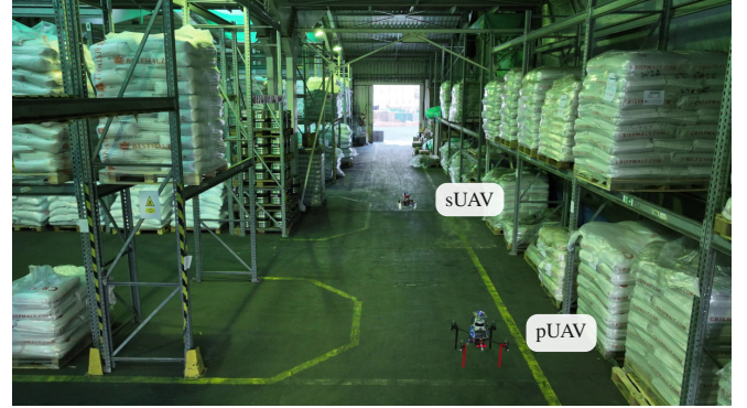
Fig. 5: Cooperative multi-UAV mapping and exploration in an industrial warehouse.
